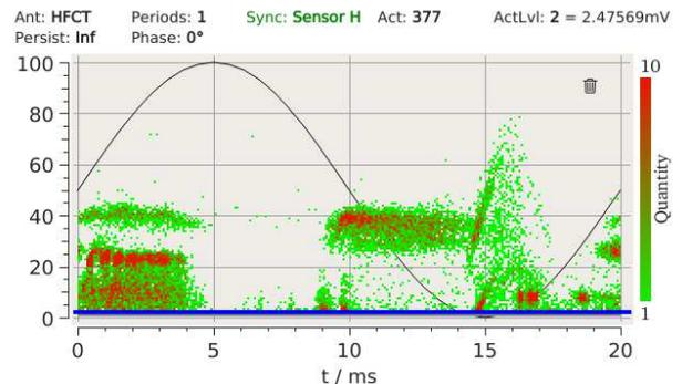
**Figure 11 PRPDP of phase L3 at HF**
