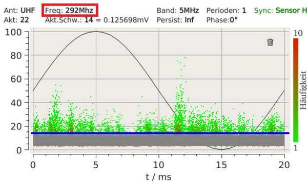
**Figure 9 PRPDP at 292MHz center frequency**
