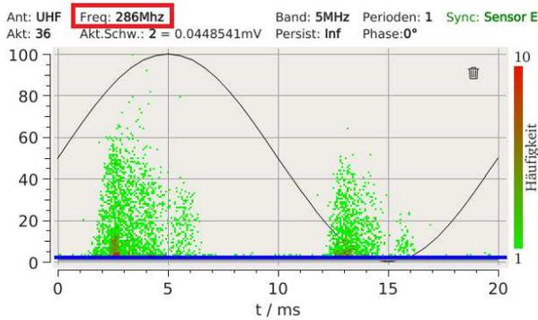
**Figure 8 PRPDP at 286MHz center frequency**
