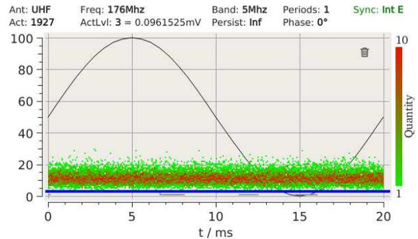
**Figure 10 PRPDP of phase L3 at 176MHz**
