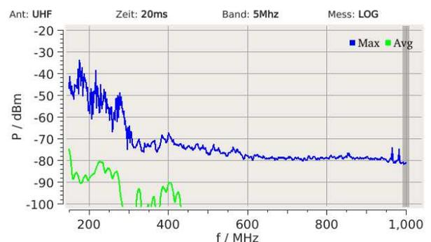
Figure 7 Spectrum discharge in large void
