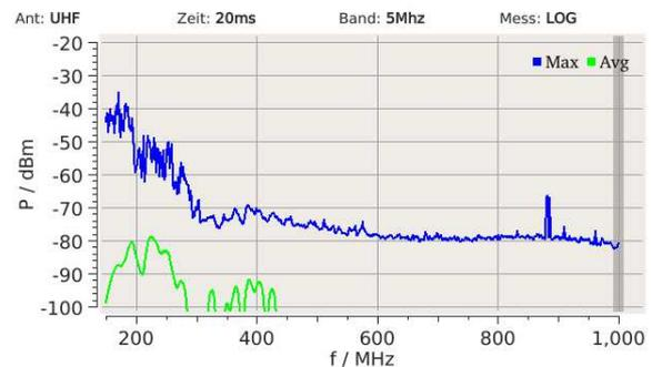
Figure 1 Spectrum of corona discharge
