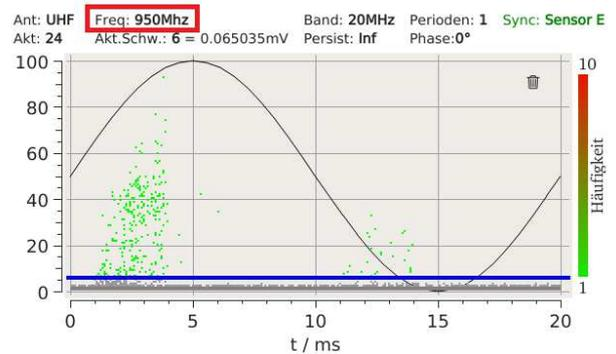
Figure 6 PRPDP at 950MHz center frequency
