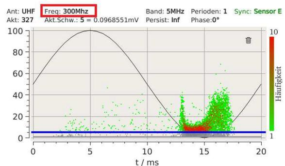
Figure 2 PRPDP at 300MHz centre frequency
