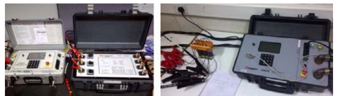
Figure - 5: Tests on the prototype transformer using the Three Phase TTR tester.
