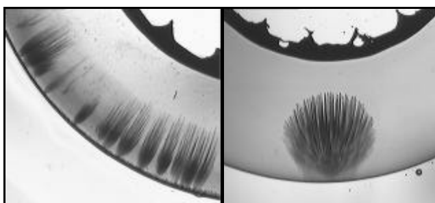
Fig. 4.2 Typical water trees found in field-aged cables. To the left, trees from a cable with tape and graphite insulation screen. To the right trees from a cable with extruded insulation screen.
